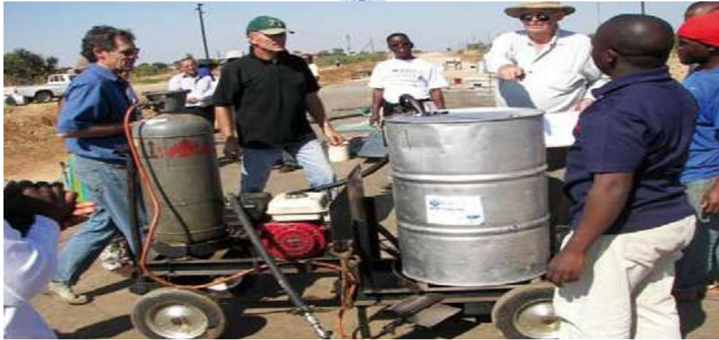
Figure2.6 Motorized hand sprayer
