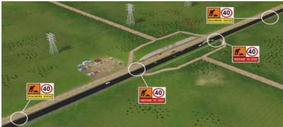
Figure.3.3 Erection of suitable road signs and warning
